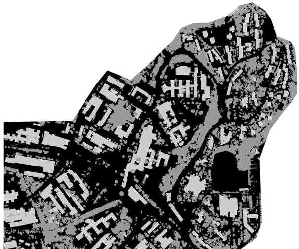
Figure 3. Classification result (Light grey: building, Dark grey: tree, Black: ground surface). The size of the subarea shown in the figure is about 1.1 km x 1.3 km.
