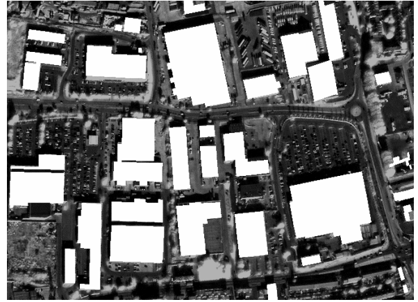
Figure 9. Final building extraction result
