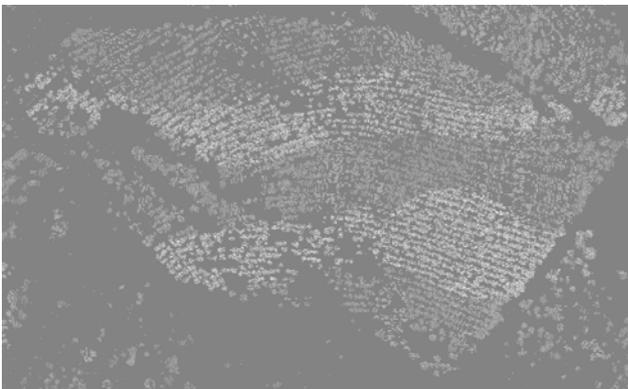
Figure 7b: stand 119 / resolution 20 cm / heights of data points between 3.5 m and 23m above ground. (3.5m – dark / 23m light) Amongst the trees are lighter and darker sections which simply mark the area of overlapping stripes. The tree height at this area does not change.
