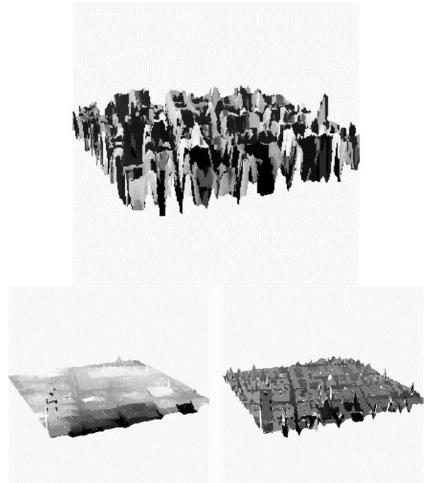
Figure 12: Three dimensional view of the original LIDAR DSM for the Piazza della Vittoria test area, together with the morphological DTM (lower left, kernel size = 25 m) and the low-pass DTM (lower right, kernel size = 100 m).
