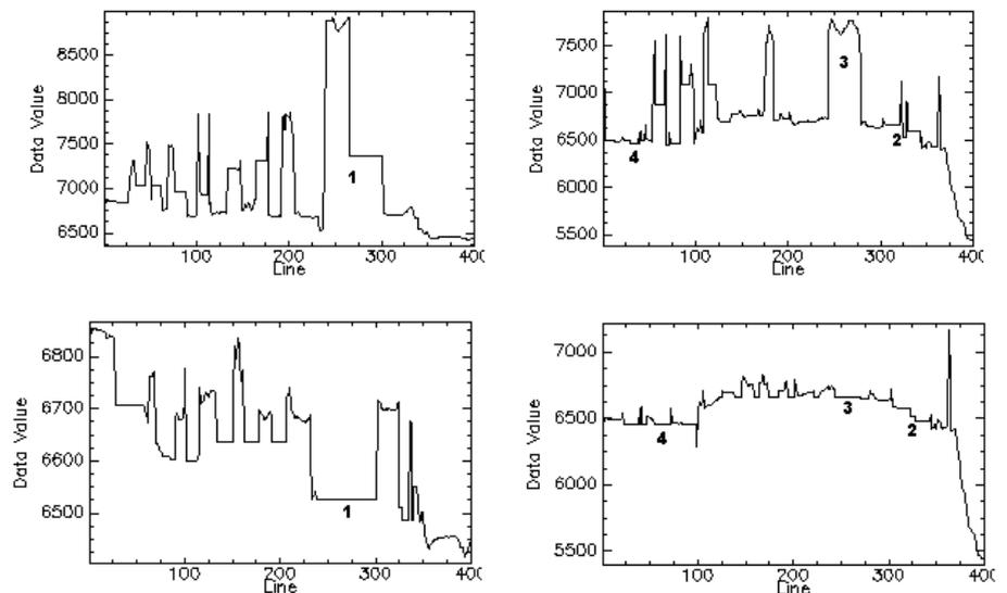
Figure 6: From top to bottom: sections Y1 and Y2 after morphological filtering with a kernel size of 10 and 100 m, respectively.
