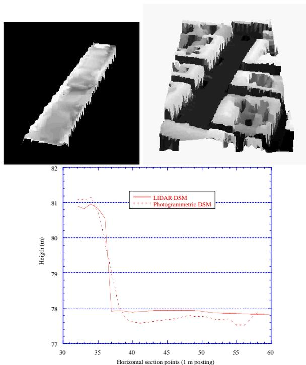
Figure.2: 3D view (on top) of the Photogrammetric and LIDAR DSM of the part of Piazza della Vittoria, where control points by analytical photogrammetry were available. Lower graph is a horizontal section of both DSMs for quantitative comparison.
