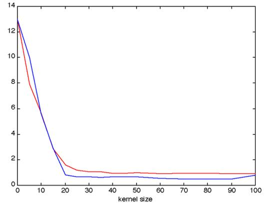
Figure 5: Mean square error between the elevation data *inside* and *outside* the buildings, computed using the data in section Y1, with respect to the filtering window width (in meters). Lower values at higher kernel sizes for morphological DTM.
