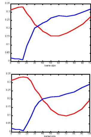
Figure 8: The absolute value of  $\bar{z}$  (decreasing curves) and  $\sigma_z$  (increasing curves) after the final low-pass filtering step applied to the first DTM approximation in figure 7 as a function of the kernel size. The upper graph refers to low-pass DTM, the lower one to morphological DTM.
