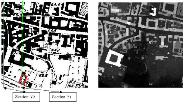
Figure.3: The raster map (on the left) and a bidimensional representation of the LIDAR height values (on the right) for the test area near the Collegio Borromeo.
