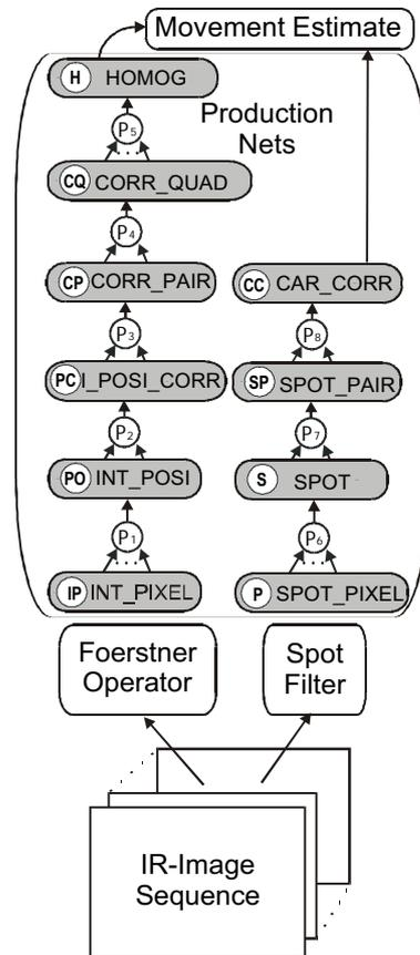
Figure 2. Production nets for GSAC-estimation of homographies and vehicle movement detection
