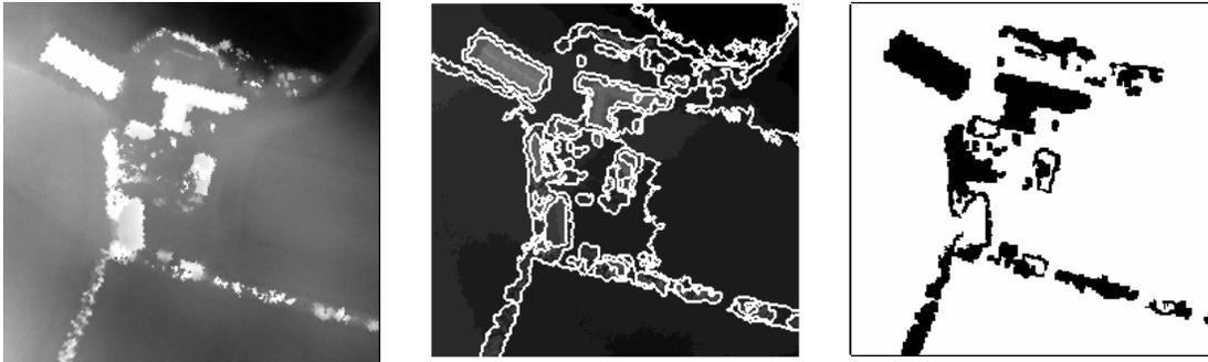
Figure 2. Given DSM (250 m • 250 m; left), results of segmentation (middle) and classification (extracted regions that have to be reduced are in black; right)
