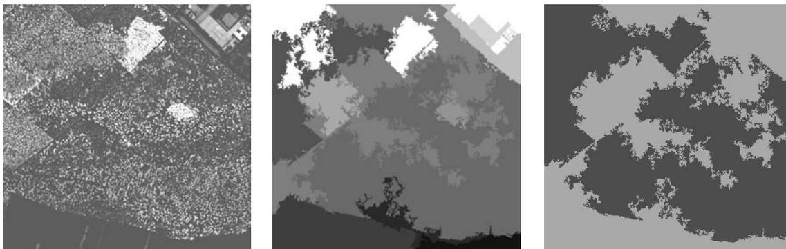
Figure 3. Given DSM (1000 m • 1000 m; left), results of segmentation (middle) and classification (extracted forest regions - not single trees - are in black; right)
