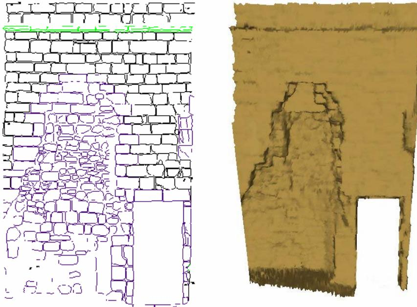
Figure 5: Left, an example of a traditional photogrammetric line plot and right, a meshed point cloud collected by a Cyrax 2400 scanner,
