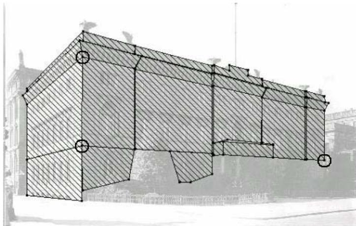
Figure 7. Manually measured points, lines, and faces.
