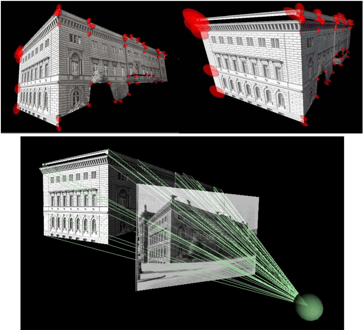
Figure 8. Top: two views of the texture mapped model, bottom: including the bundle of rays and the original image.
