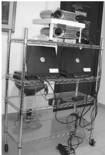
Figure 1: Set-up for our mobile virtual environment. From top to bottom: the two video projectors with their polarized filters and the two laptops. The computers are interconnected with a twisted wire.
