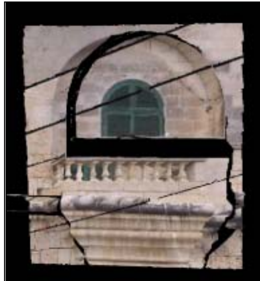
Figure 1: Scan lines appear between one line of photos and another as is evident in this figure and in Figure 2 (next page).
