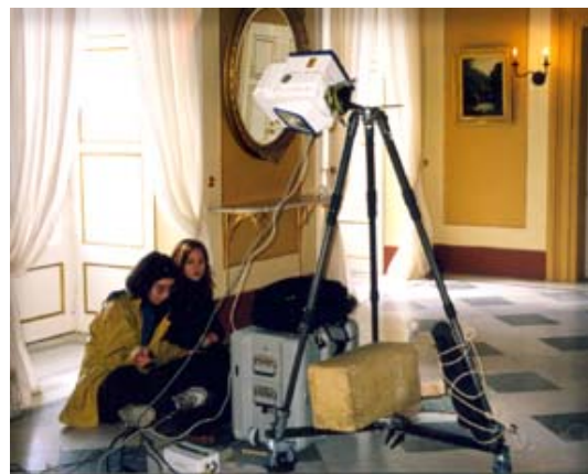
Figure 7: GS Scanner in bay 5, placed in a horizontal position
