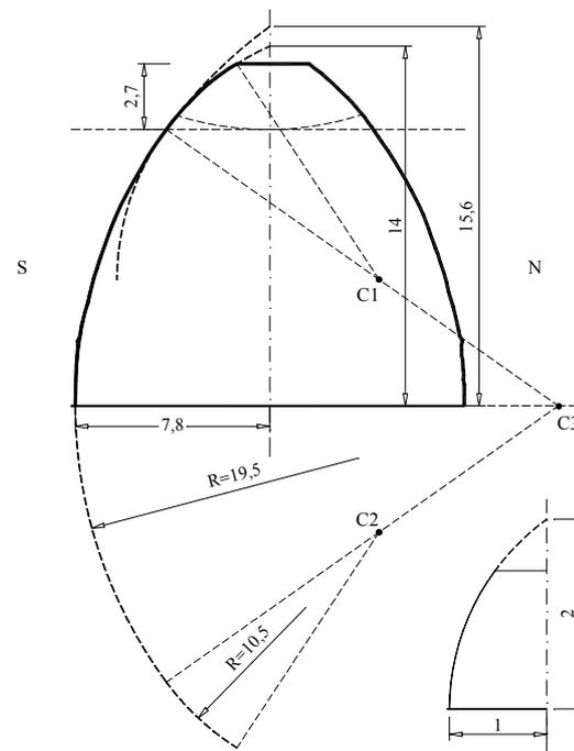
Fig.13-Comparison of the section N.S with the tricentric curve
