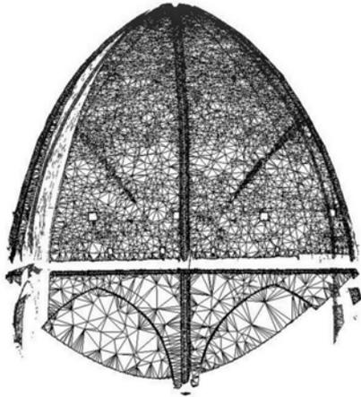
Fig. 10-The mesh created by the aggregation of the points.
