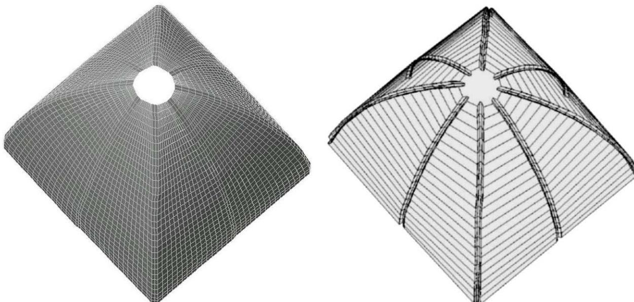
Fig.18-geometric Model and mesh for the calculation.
