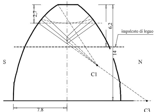
Fig. 17- Vertical section with indication of the possible building technique.
