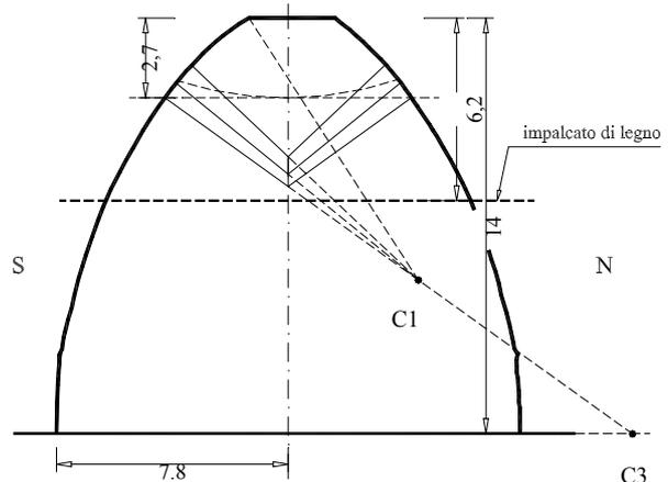
Fig.17- Vertical section with indication of the possible building technique.
