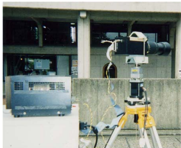
Figure 1. CCD Line Sensor System used in this study
