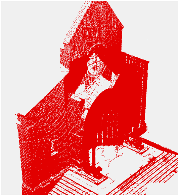
Figure 1. All points acquired by Mensi GS100 laser scanning
