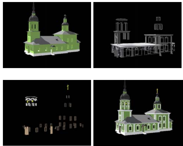
Figure 1: Structured VRML model. Top left: LOD 0, top mid-right: supplement to LOD 1, down left: supplement to LOD 2, down right: complete model containing all three sub-structures.
