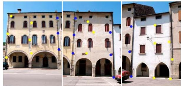
Figure 7: CCD static images of contiguous façades to be rectified by MMS surveyed control points.
