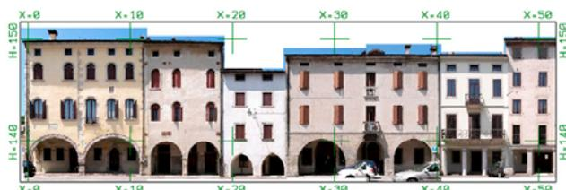
Figure 10: Joining of previous rectifications (1:600 scale).
