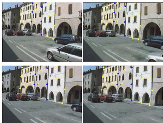
Figure 5: 3D-survey of control points by means of four consecutive MMS images.
