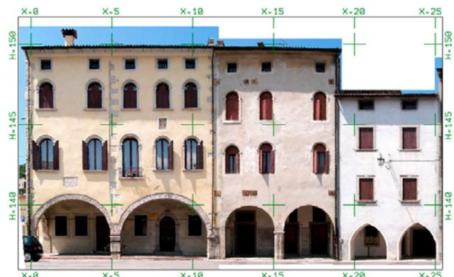
Figure 8: Previous CCD static images rectified (1:300 scale).
