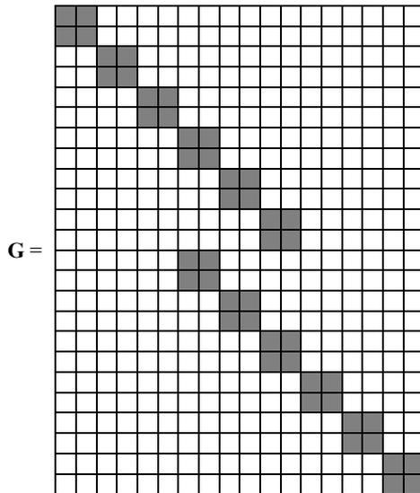
It is now clearest how in matrix  $G$ , 7th÷18th rows link the images in a unique solution or, conversely, 7th÷12th columns submit the common points to two homographic constraints.
