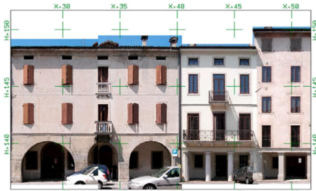
Figure 9: Other CCD static images rectified (1:300 scale).
