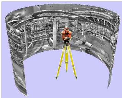
Figure 3. The Hazmap camera and a partial panorama generated from multiple image tiles.
