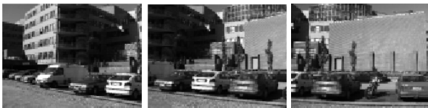
Figure 11. A block of three concentric images used for the camera calibration. The horizontal overlap between these images is 50%.
