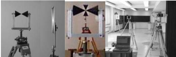
Figure 4. The practical arrangement for mounting the camera consists of vertical and horizontal targets (left). When joint in line, the targets appear as symmetric cross and free from parallax as seen from the camera (middle). The set up for camera mounting is arranged in one horizontal plane (right).
