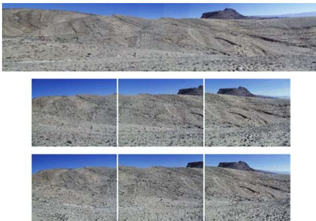
Figure 13. A panoramic stereo view (4707 x 1000 pixels, 120° x 40°) built from the three images in the second row. The images in the third row belong to the left image of the stereo pair. The base of this stereo photography is 13 meters and the distance to the road on the opposite slope about 120 meters. The size of a single frame is 1280 x 1024 pixels (50° x 40°).
