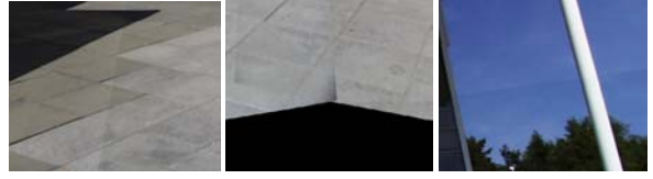
Figure 8. Details of the joints between transformed images. The radiometric differences allow a gross visual check of the transformation. All linear edges crossing the joints should appear as linear in the composition.
