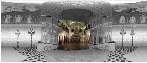
Figure 7: Panoramic image data have been fused in a sub-window of the shown range image. (The figure shows the Thronsaal of castle Neuschwanstein.)
