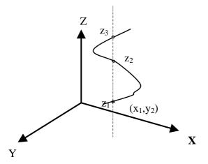
3D Modelling (Raper, 2000): 3D modelling is the ability to assign up to three z(height) values to a point (see figure above).
