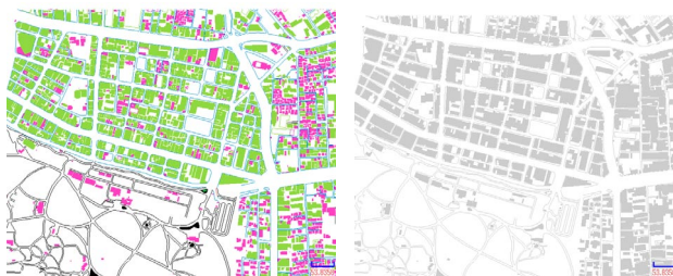
Figure 8. Generalized result: Original buildings and roads (up: 1/2500) and aggregated buildings and simplified roads (down: 1/25000)
