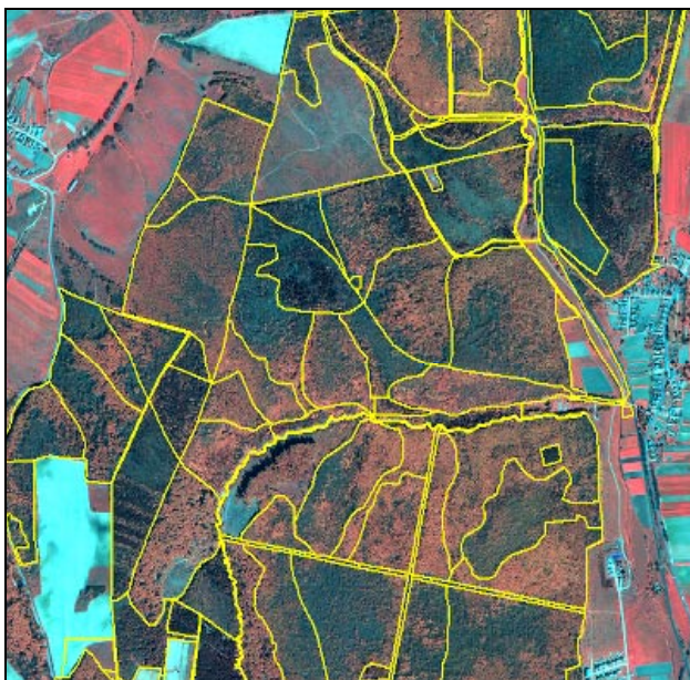
Figure 1. One part of the research area. False colour composite (R: Ikonos NIR band, G: Ikonos green band, B: Ikonos blue band). Orthorectified image with digital forestry map database polygons. Image copyright Space Imaging 2001. Image resolution was digitally degraded.
