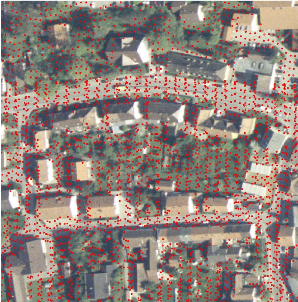
Figure 5. Digital orthophoto overlaid with LIDAR measurements
