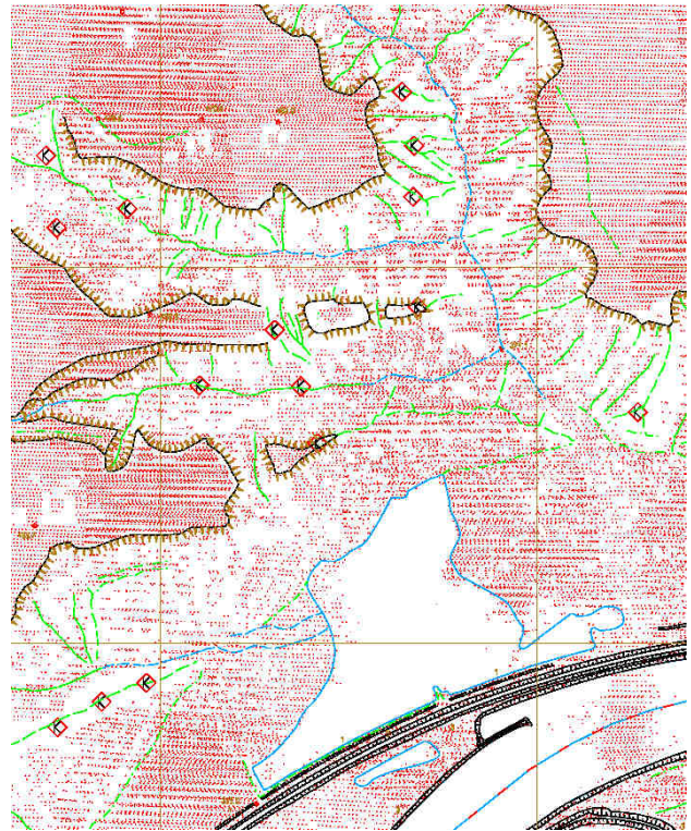
Figure 2. Point plot of LIDAR points overlaid with morphological features and markers for field check
