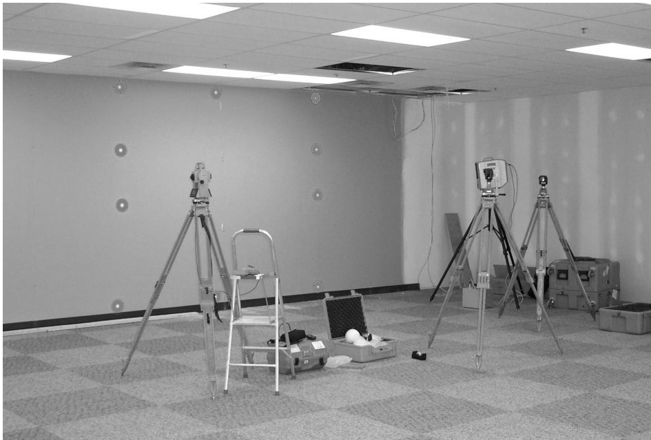
Figure 1: Set-up for Scans of the Wall
