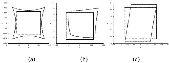
Figure 4. Distortions in box-type configuration: radial distortion (a), decentering distortion (b), and Affine deformation (c).
