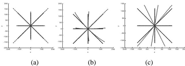
Figure 5. Distortions in X-type configuration: radial distortion (a), decentering distortion (b), and Affine deformation (c).
