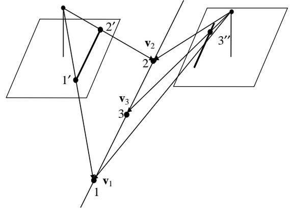
Figure 1. 3-D straight lines in frame camera imagery.
