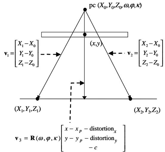
Figure 2. Mathematical model for including straight lines in frame camera imagery.
