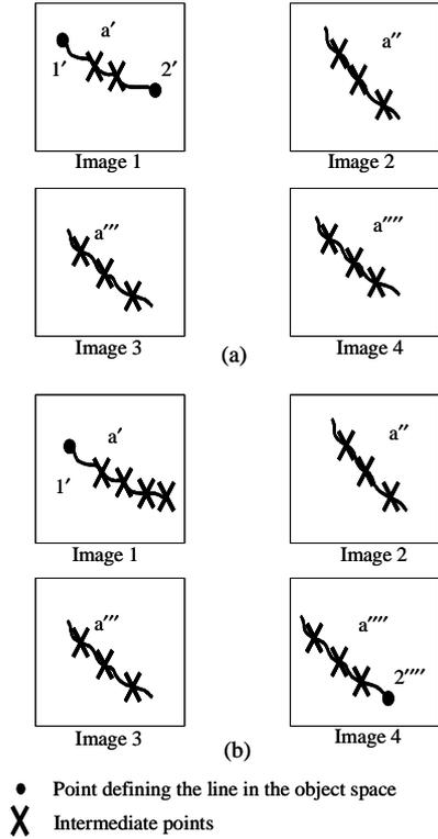
Figure 3. Schematic drawing representing two scenarios for the selection of the end and intermediate points in overlapping images.
