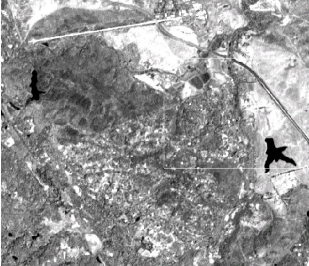
**Figure 3.** Landsat 7 panchromatic image. Rendering visible and very near infrared reflectance at 15 meters ground resolution. The area shown is the same as in Figure 2. White box indicates coverage of Figure 4.
