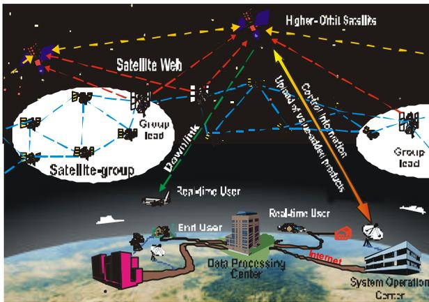
Figure 2. The architecture of a future EO satellite system
