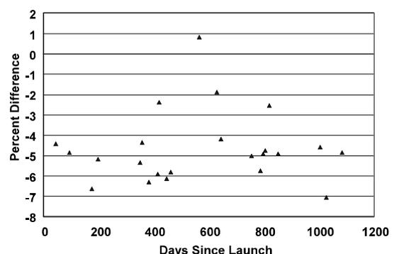
**Figure 1.** Percent difference between vicarious and preflight results for Band 1 of ETM+ for all data sets collected by RSG.
