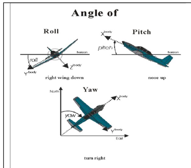
Figure 1: Definition of roll, pitch and Yaw conform to ARINC 705
