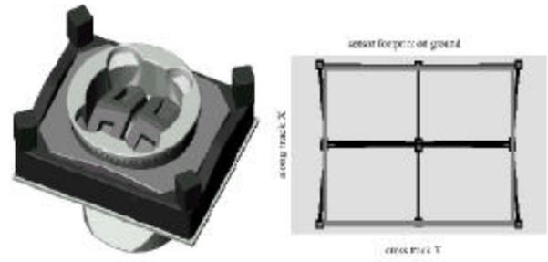
**Figure 6:** The DMC by Z/I Inc consists of 4 independent camera cones to build one large image, and additionally 4 cones to add color in red, green, blue and infrared. Each of the color images is at a fraction of the resolution of the panchromatic images. From the 4 individual images a “virtual image” is built (Source: Z/I inc., 2002).
