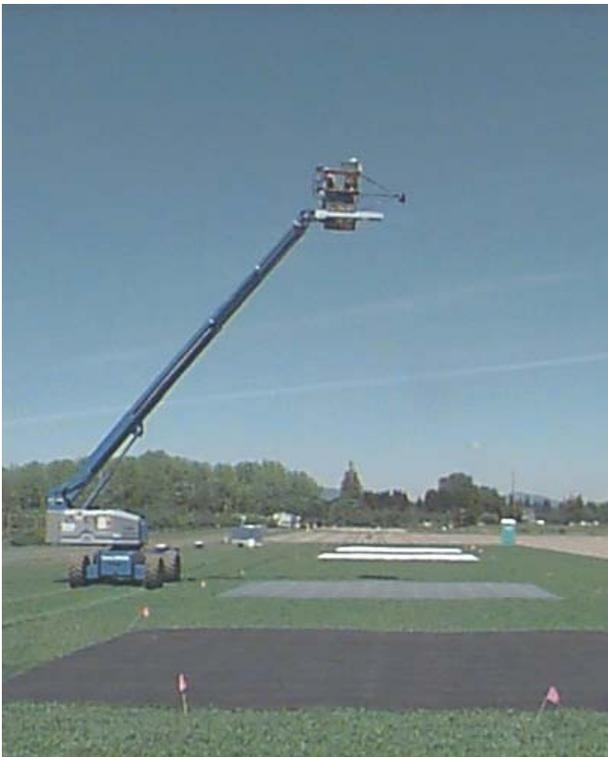
Figure 2. Boom-mounted spectral measurement system.
