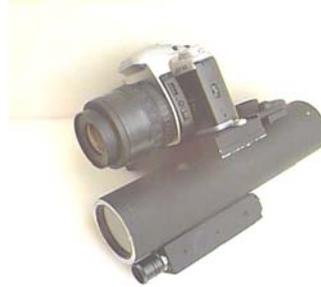
Figure 3. Baffled tube foreoptic with film and video cameras.
