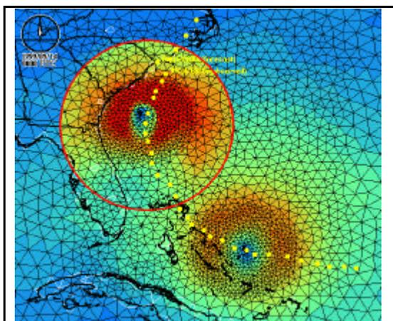
Figure 1. Dynamic grid adaptation puts high resolution only where needed, leading to the accurate and computationally efficient prediction of high wind speed (color) and track of hurricane Floyd. The initial conditions are shown with an inset showing the high-resolution area at 48 hours into the forecast. The yellow dots show the observed storm track.
