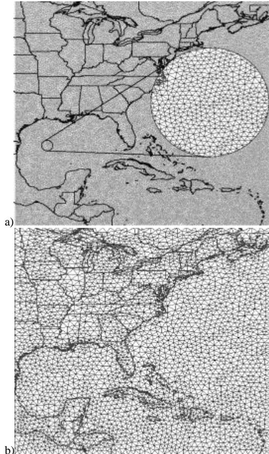
Figure 3. OMEGA domain and grid for (a) the baseline high-resolution and (b) coarse resolution control run.
