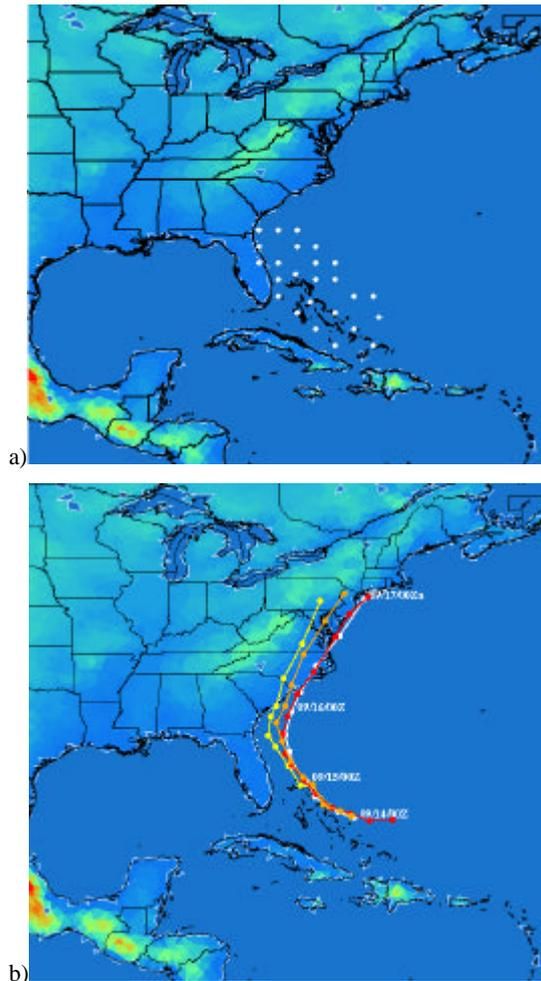
Figure 6. a) The location of 25 pseudo-soundings that have extracted from the control run, b) OMEGA forecasted hurricane Floyd track for this adaptive observation run (orange) as compared to the observed track (white), the control run track (red), and the coarse resolution run (yellow).
