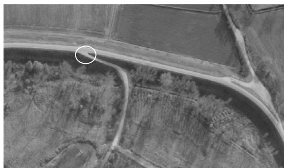
Figure 8. Point on a elevated road in which the differences between GPS and LIDAR heights are higher than 1 m.
