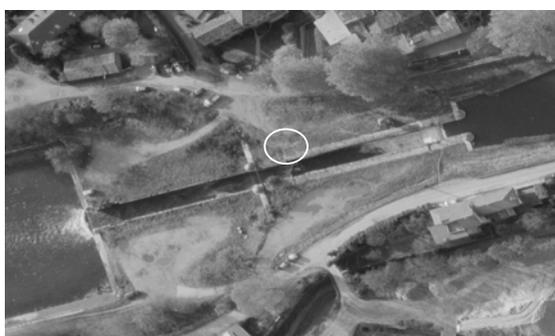
Figure 9. Point on an embankment in which the differences between GPS and LIDAR heights are higher than 1 m.
