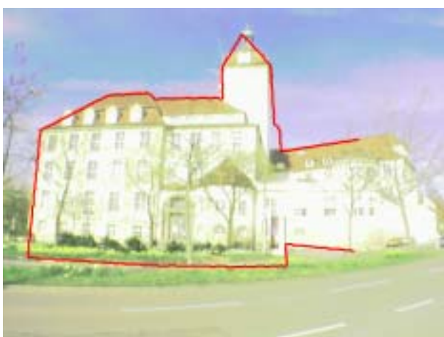
Figure 9. Building localization based on Generalized Hough Transform. Top image shows the 3D model projected by measured orientation, bottom depicts the detected silhouette .
