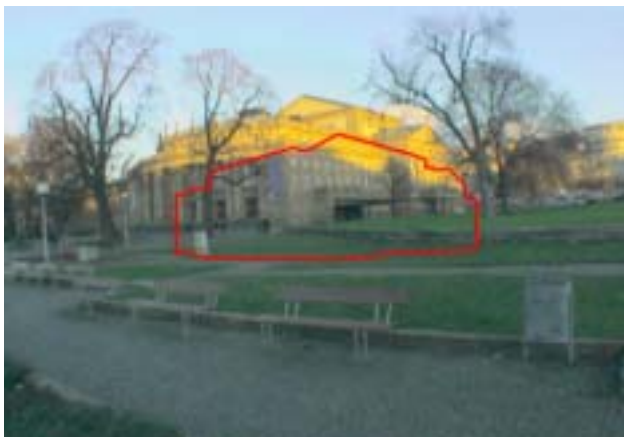
Figure 4. Silhouette of the building as projected to the image based on the exterior orientation from GPS and digital compass.
