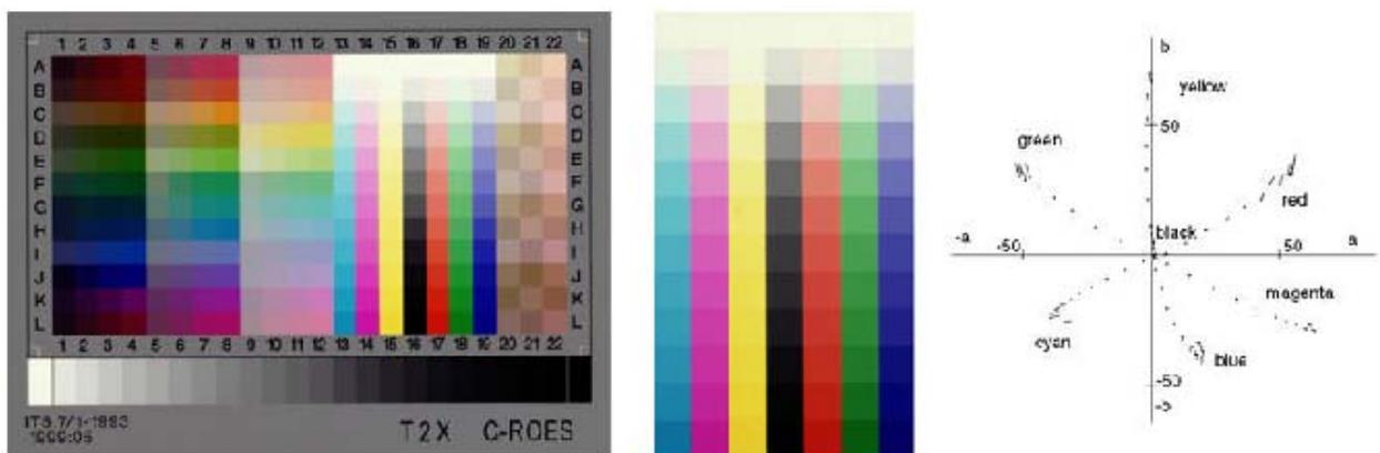
Figure 5. The IT8 color calibration target is used control the radiometric performance of a scanner. Left: full target, showing 246 color tags and 24 greyscale tags. Middle: scale of the 6 primay colors and black. Right: Transform of measured color values and reference values.
