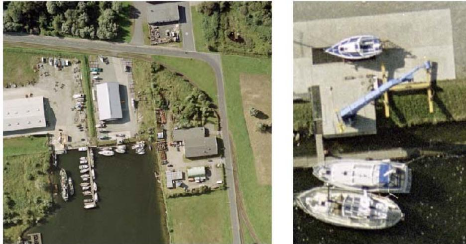
Figure 7. Aerial image at scale 1:5000. The AGFA X100 color negative film shows a remarkably fine granularity and allows scanning at a resolution of 2500 dpi
