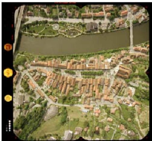
Figure 2. Aerial image, 23 mm by 23 mm results into a digital file of several hundred megabyte of data (e.g. 705 MByte @ 15  $\mu$ m pixel size and 3 by 8 bit color depth)
