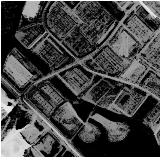
Figure 4. Extracted road networks in the industrial area depicted in Figure 3 (long bright linear objects are road networks).
