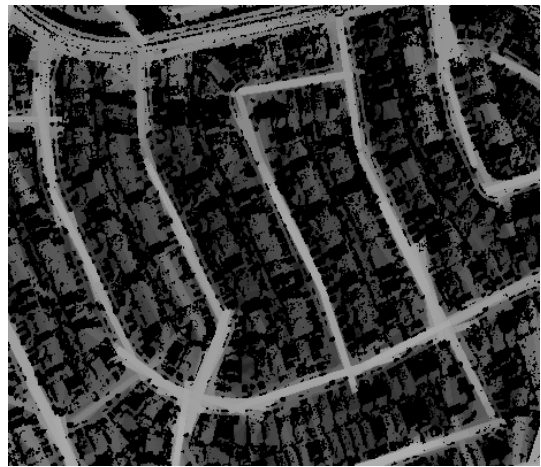
Figure 2. Extracted road networks in the residential area depicted in Figure 1 (long bright objects are road networks).
