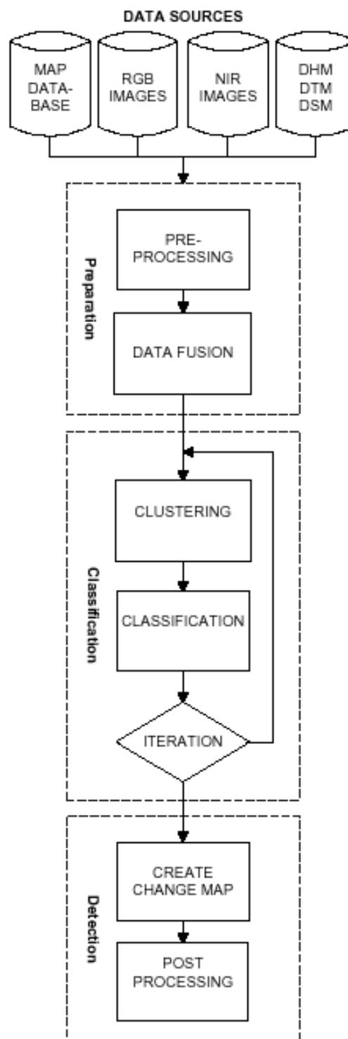
Figure 2. Change detection work flow—cf. section 3 for description
