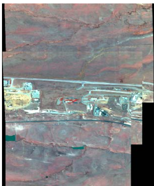
Figure 4. Mosaicked rectified images with the original exterior orientation parameters
