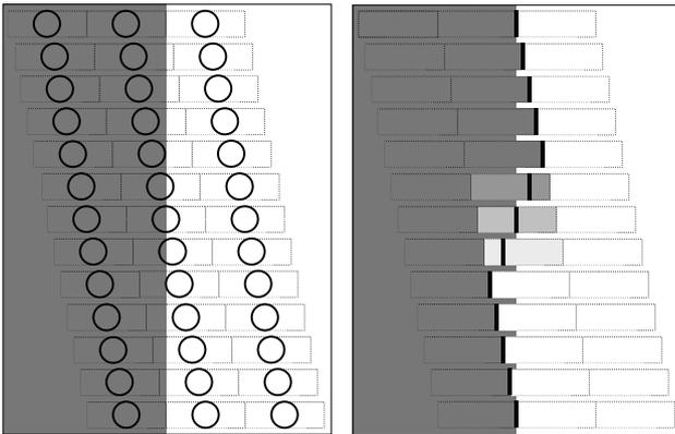
Figure 6: Left: footprints on scan lines across a grey value edge. Right: resulting pixel grey values and reconstructed edge locations. See text.
