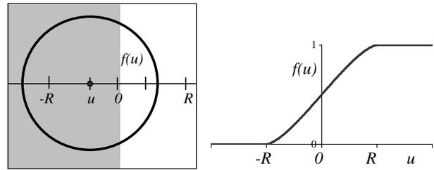
Figure 7: (a) Footprint located at unsigned distance  $u$  from a grey value edge. (b) Fraction of footprint on bright side of the edge.
