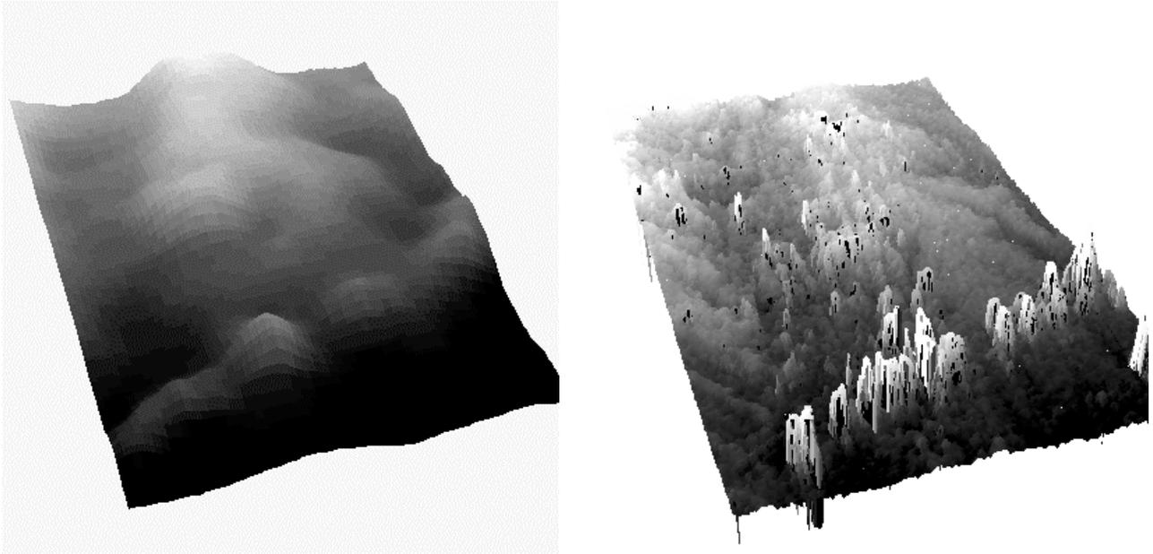
Fig. 1: Three-dimensional visualization of the DEM of the UCLA and Wilshire Boulevard area in Los Angeles: SRTM and TOPSAR data are shown on the left and right, respectively.
