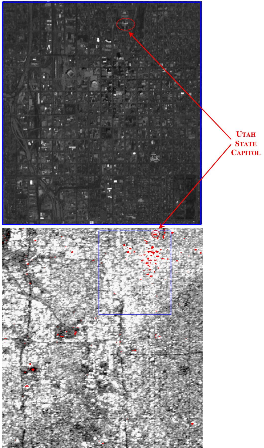
Fig. 4: Results of the analysis in the Salt Lake City area: on top, the 10 m SPOT image provided by NIMA and used as ground truth; on bottom, the SRTM magnitude image with superimposed red blobs depicting the buildings detected in the area.
