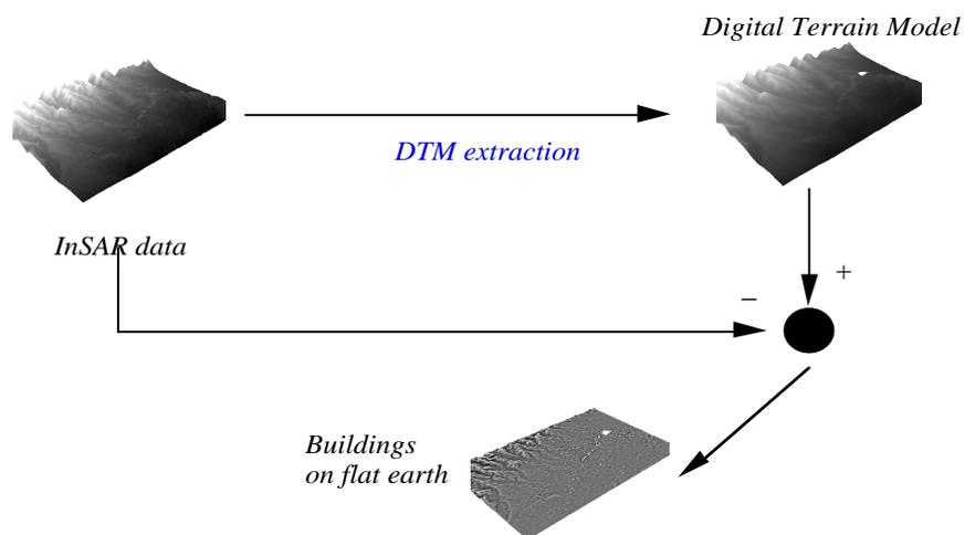
Fig. 2: The overall structure of the procedure used to analyze SRTM height data.
