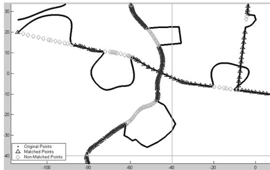
Figure 4. Example of detected changes between road segments in image and object space.
