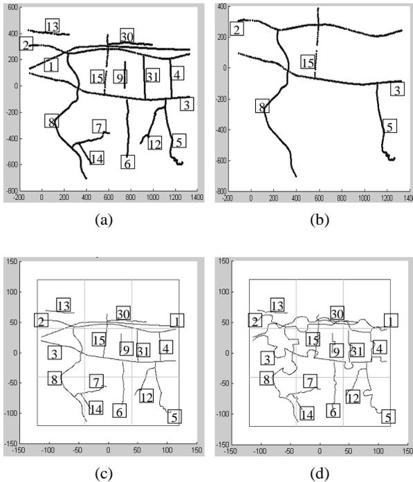
Figure 3: Object space linear features O1 (a), and O2 (b), and image space linear feature without digitisation errors I1 (c) and with digitisation errors I2 (d). Roads are labelled for further references.
