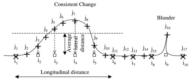
Figure 2: Consistency check between the object and image data points. The rectangular points with labels  $i_1$  to  $i_{10}$  are the projected object space points along a linear feature into the image space, while the crosses with labels  $j_1$  to  $j_{17}$  are the points along the corresponding linear feature in the image space.
