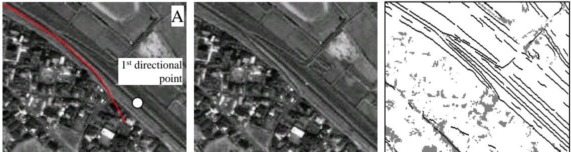
(b) Enlarged figure of area "A", (Left #1: result of road line extraction, Left #2: IKONOS image, Right #1: road mask and road seeds).
