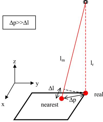
Figure 1. Tie-point position error and its influence on the coordinate components
