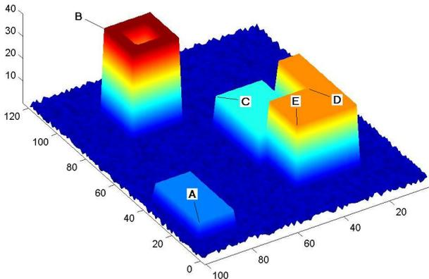
Figure 3: The virtual scenery created for the simulations and the tie-points (A, B, C, D, E) used for the global registration
