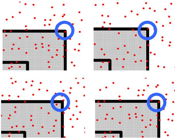
Figure 4. Particular of the distribution of the laser footprints around the corner of one building (tie-point B) in four different scans.
