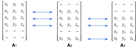
$$\begin{aligned} \text{diag}(\mathbf{M}_1) &= [1 \ 1 \ 1 \ 1 \ 0 \ 0]; \\ \text{diag}(\mathbf{M}_2) &= [0 \ 1 \ 1 \ 1 \ 0 \ 1]; \\ \text{diag}(\mathbf{M}_3) &= [0 \ 0 \ 1 \ 1 \ 1 \ 1] \end{aligned}$$
