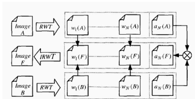
Figure 1. Scheme of the multisource image fusion algorithm proposed in (Chibani & Houacine, 2000).
