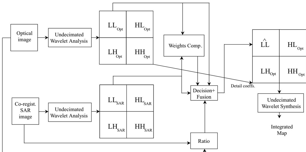
Figure 2. Scheme of M-UDWT.
