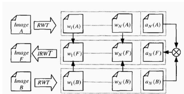
Figure 1. Scheme of the multisource image fusion algorithm proposed in (Chibani & Houacine, 2000).
