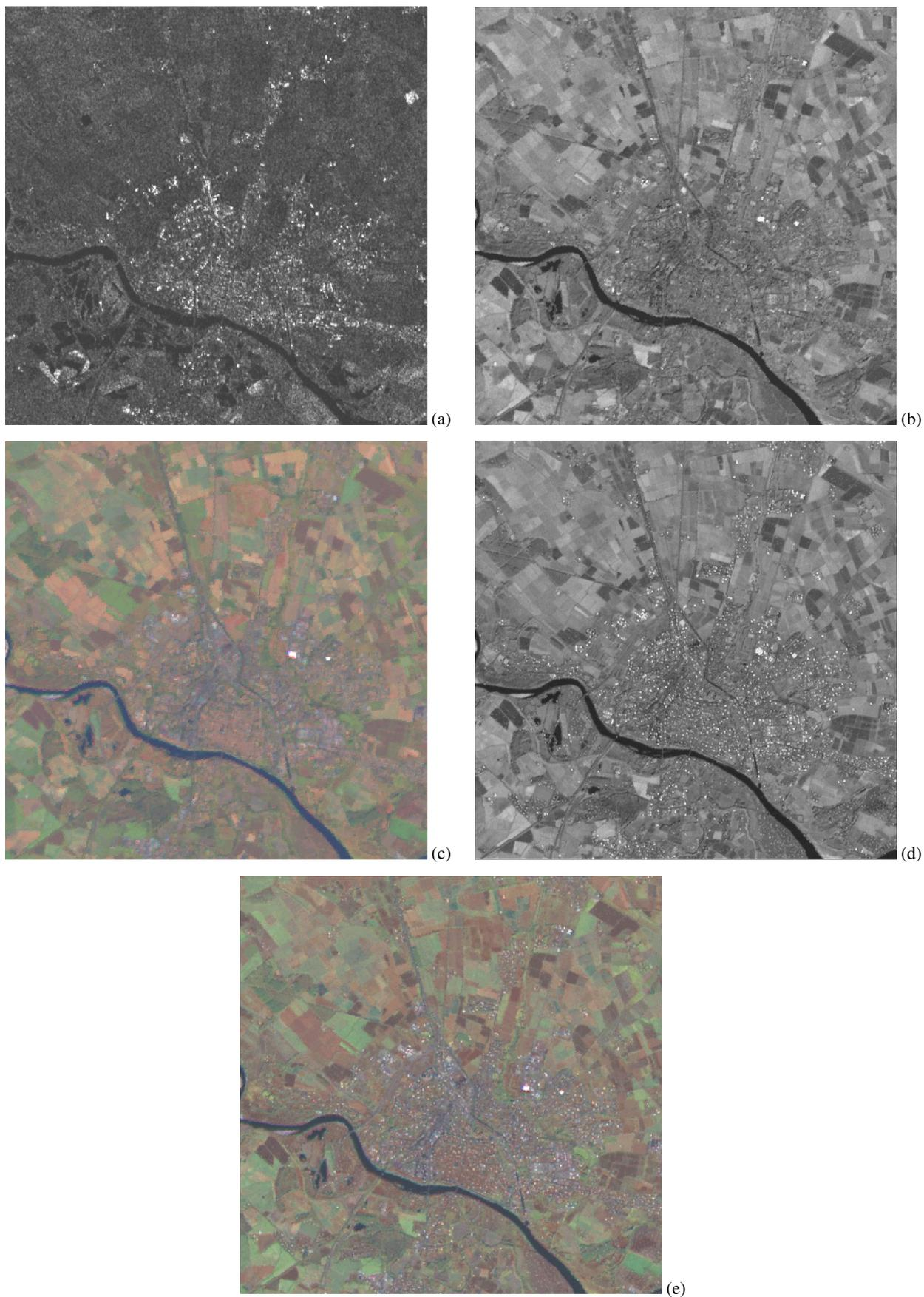
Figure 3. (a): Radarsat image, Pavia, Italy; (b): Landsat 7 panchromatic image; (c): Color composite ( $R=B5$ ,  $G=(B4+B3)/2$ ,  $B=(B2+B1)/2$ ) of original MS data; (d): Integrated map P+SAR; (e): Color composite of integrated MS+SAR data.
