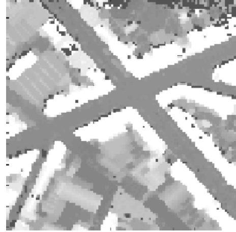
Figure 8: The Digital Elevation Model used as a reference. The black values correspond to pixels where altitude values are not determined
