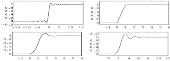
Figure 6. Four examples of the error function generated by different low-pass filter which is the ideal low-pass filter (upper left), Haar scaling function (upper right), Asymmetric Daubechies scaling function of order  $N=3$  (lower left), and  $N=10$  (lower right), respectively (Tsay, 2000)
