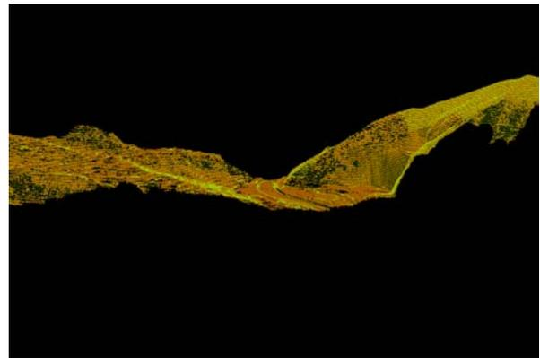
Figure 6: DTM generated from laser scanner data.
