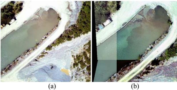
Figure 12: Lake Surface in the generated Orthophoto (a) using OrthoEngine Software (b) using TerraPhoto software.
