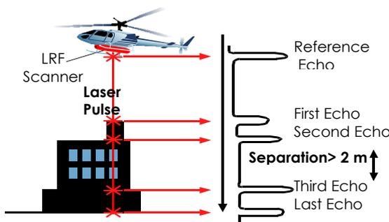
Figure 1 Laser Survey Principle (TopEye System, [www.topeye.com](http://www.topeye.com))
