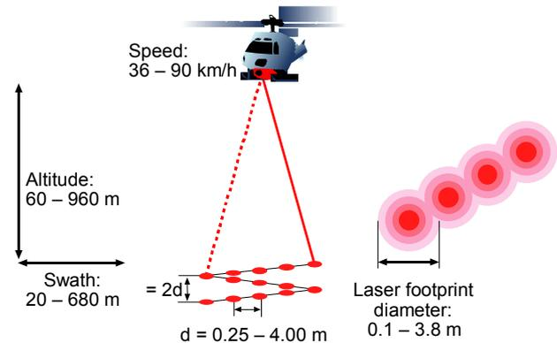
Figure 2 Laser Survey Principle Principle (TopEye System, [www.topeye.com](http://www.topeye.com))
