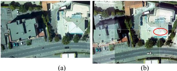
Figure 12: Edge matching in the generated Orthophoto (a) using OrthoEngine Software (b) using TerraPhoto software.
