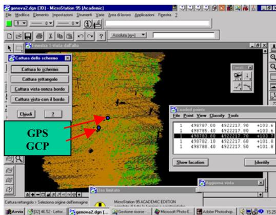
Figure 5: The two GPS ground control points on top of the generated DSM.
