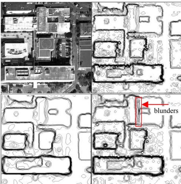
Figure 6: GSI matching results; top-left: image window that covers a city area with rich texture; top-right: contours derived from the G\_Rex matching results; bottom-left: result from G\_Rex+GCMM; bottom-right: result from G\_Rex+F\_MPGC; contour interval: 0.5 m
