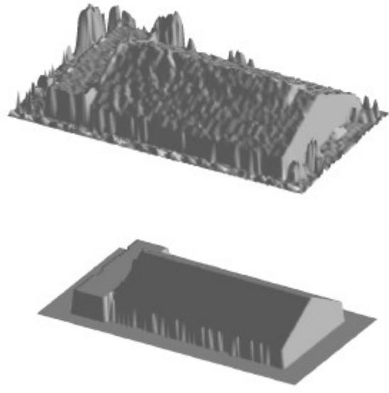
Figure 6. The Original and Refined DEM for Building 2
