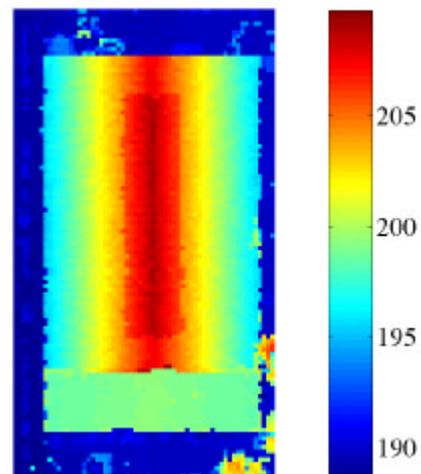
Figure 2-c. The Elevation Shaded LIDAR DEM (Building 2)
