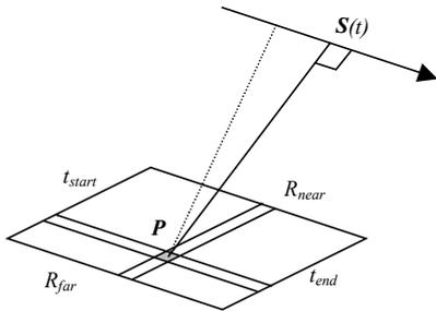
Figure 3 - Point being imaged in a SAR image processed at zero Doppler
