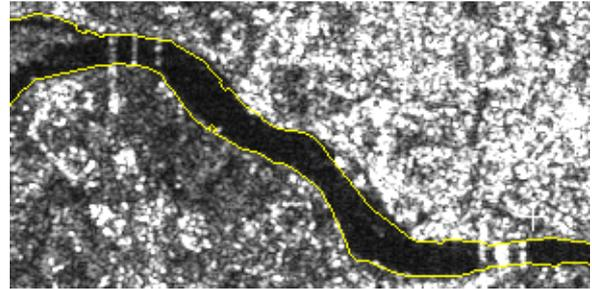
Figure 4 - Portion of an ERS-1 image (300 by 150 pixels) with superimposed vector data corresponding to the river margins, projected onto the image space.
