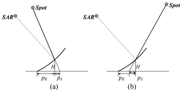
Figure 6 – Same side (a) and opposite side (b) configurations in a SAR-SPOT stereopair.
