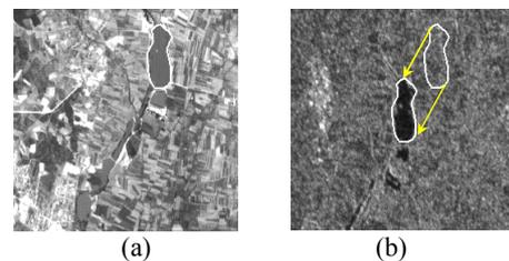
Figure 9 – Determination of tie-points using area features.
