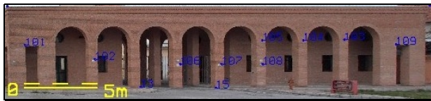
Figure 11: CCD rectified image (here plotted at 1:350 scale).
